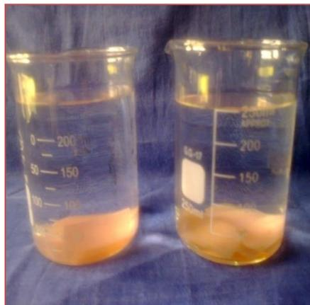
**Figure (8):** 10 Samples of heat cured acrylic & 10 samples of flexible resin are immersed in synthetic saliva alone as a control.
