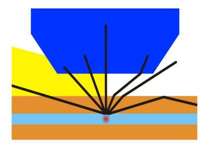
Oil immersion increases the resolving power of the microscope by replacing the air gap between the immersion objective lens and cover glass with a high refractive index medium and reducing light refraction
