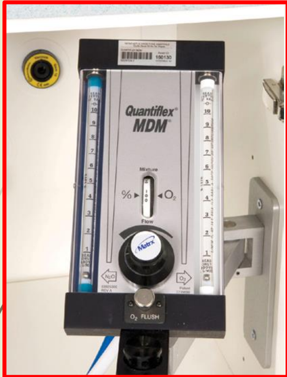
1- flow control head, showing nitrous oxide and oxygen flow meters, mixture control dial, flow control knob and oxygen flush button.
