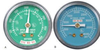
• Fig. 6.20 Pressure gauges on tanks containing (A) oxygen and (B) nitrous oxide require different interpretations of how much remains in the tank. When an oxygen tank is full, the gauge shows the actual psi of the oxygen remaining in the tank. However, for nitrous oxide, the psi represented on the gauge only represents the pressure of the N_2O vapor floating above the liquid N_2O . It is only when the amount of liquid begins to run out that the psi on the N_2O gauge begins to fall below 750 psi. Until that time, the gauge will read 750 psi.
