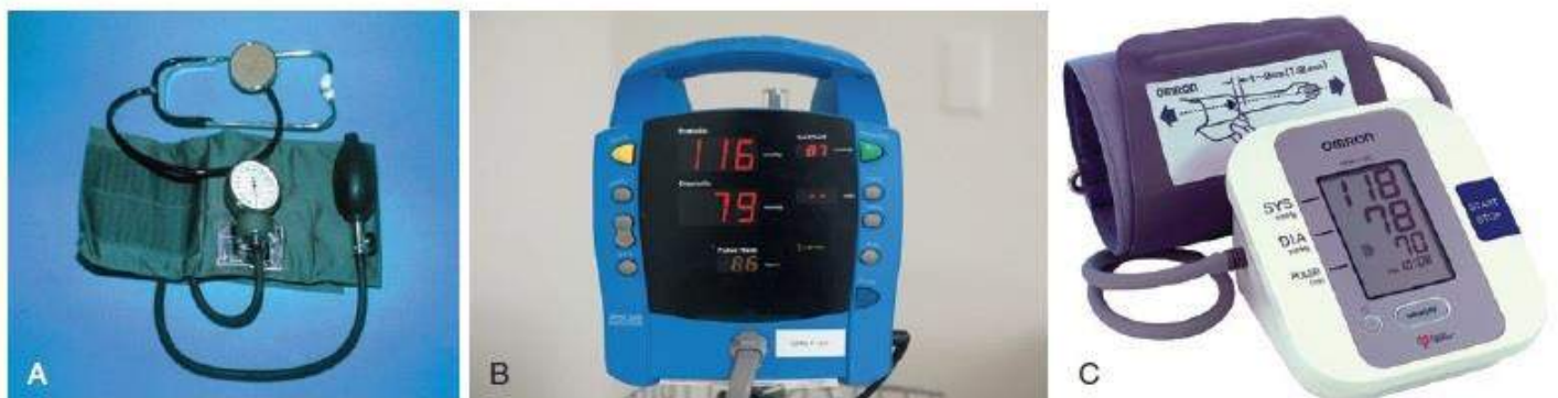
FIG 1 (A) Standard blood pressure cuff (sphygmomanometer) and stethoscope, (B) and (C) automated blood pressure devices.
