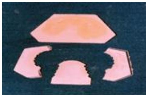
Fig.(14):- Stone parts of the upper half of flasking before forming the mold.
