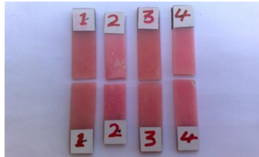
Figure 1: Specimens were cut surfaces parallel to each other
