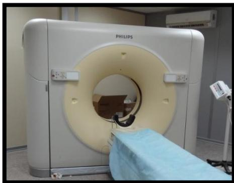
Fig.(1):- Multi-slice computed tomography machine (PHILIPS Brilliance 64) used for analysis of the specimens.
